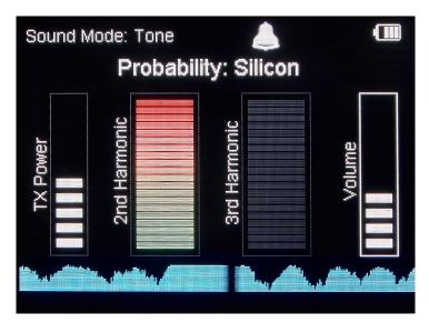
Main Screen with detected signal on 2nd Harmonic
