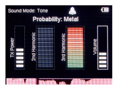
Main Screen with detected signal on 3rd Harmonic
